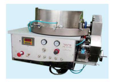
Automatic tablet printing machine can print characters on any tablets in any size and shape like round, ovals, triangular, hexagonal tablets. Feed disc & gravure rollers are available in any size in order to obtain most efficient production. It is compact in structure and easy to operate. Scrapping of excess ink on the printing roller is done on the pneumatic pressure or manually.
